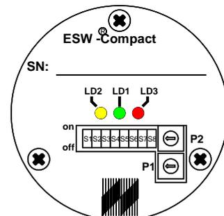
Upon execution of the self-test function, it's absolutely necessary to return the switch S8 to the position OFF in order to ensure the proper function of the ESW<sup>®</sup>-Compact/Ex. The yellow LED must darken and current has to return to his normal value. In case the yellow LED is lighting and a higher output current is flowing, without of activation of S8, than the electronic recognize one sensor defect and starts alarm, because the electronic is continuously monitoring the sensor.
