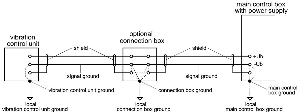
If an isolated installation is not specially requested, usually through the attachment with screws each case is connected to the local machine ground.
