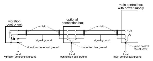
If an isolated mounting is not explicitly desired, it can usually be assumed, by screwing the components together, that the housings will accept the respective local machine ground potential.
